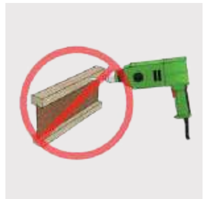
Do not drill the flange
