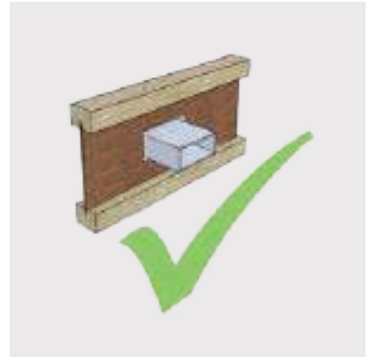
Do run MVHR through the web
